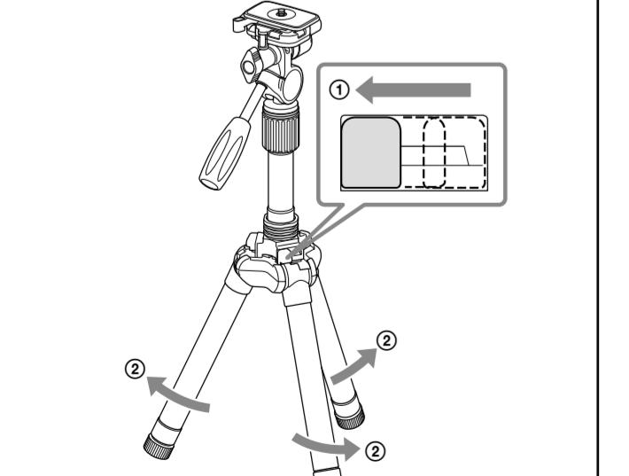
Return the set-up/storage mode switch (A-8) to storage mode by lifting and turning it. (Do this step with the legs closed as illustrated.)
