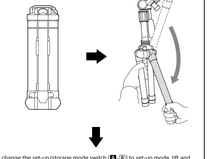
To change the set-up/storage mode switch (A-8) to set-up mode, lift and turn it until the white dot is aligned with the white line. (Do this step with the legs closed as illustrated.)
