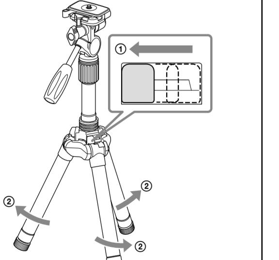
Set the leg opening stopper (A-9) of each leg to the left position, and close the legs. Leg opening angle: Approx. 24° in the left position, Approx. 45° in the center position, Approx. 75° in the right position.
