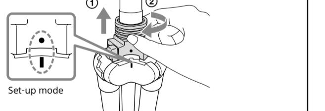
Make sure the leg opening stopper (A-9) of each leg is in the left position, and open the legs. Leg opening angle: Approx. 24° in the left position, Approx. 45° in the center position, Approx. 75° in the right position.
