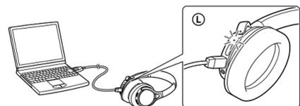
When the unit and the computer are connected, charging starts and the indicator (red) lights up. Charging is completed in about 2.5 hours at most and the indicator (red) goes off automatically.
